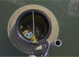
This summer, Harbour West Marina installed a new Seabin to collect floating litter in the marina area. The device works by suctioning surface water and debris down through a catch bag, holding any litter and plastics so they can be disposed of properly. The Seabin was hard at work through the end of boating season, catching food wrappers, plastic bottles, and many cigarette butts.
