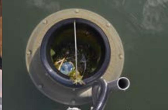
This summer, Harbour West Marina installed a new Seabin to collect floating litter in the marina area. The device works by suctioning surface water and debris down through a catch bag, holding any litter and plastics so they can be disposed of properly. The Seabin was hard at work through the end of boating season, catching food wrappers, plastic bottles, and many cigarette butts.
